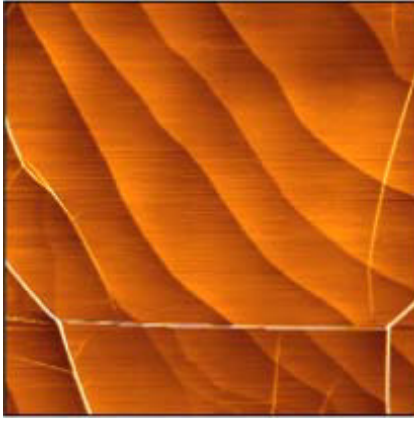
Figure 16. A 8\mu\text{m} \times 8\mu\text{m} AFM image of a 10–12 layer graphene film grown on the SiC(0001) C-face in a furnace environment [108]. Lines are ‘puckers’ in the graphene similar to those shown in figure 12.
